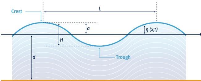
Characteristics of a 2D linear water wave
